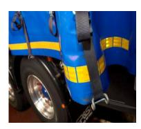
We offer a complete range of 3M ECE104 homologated retroreflective safety markings for rigid and curtain sided vehicles.
