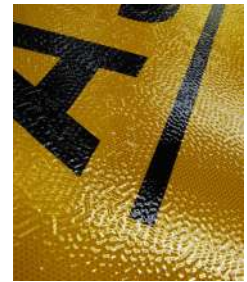
Water damage caused by storing signs outdoors in transportation packaging.
