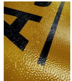
Water damage caused by storing signs outdoors in transportation packaging.
